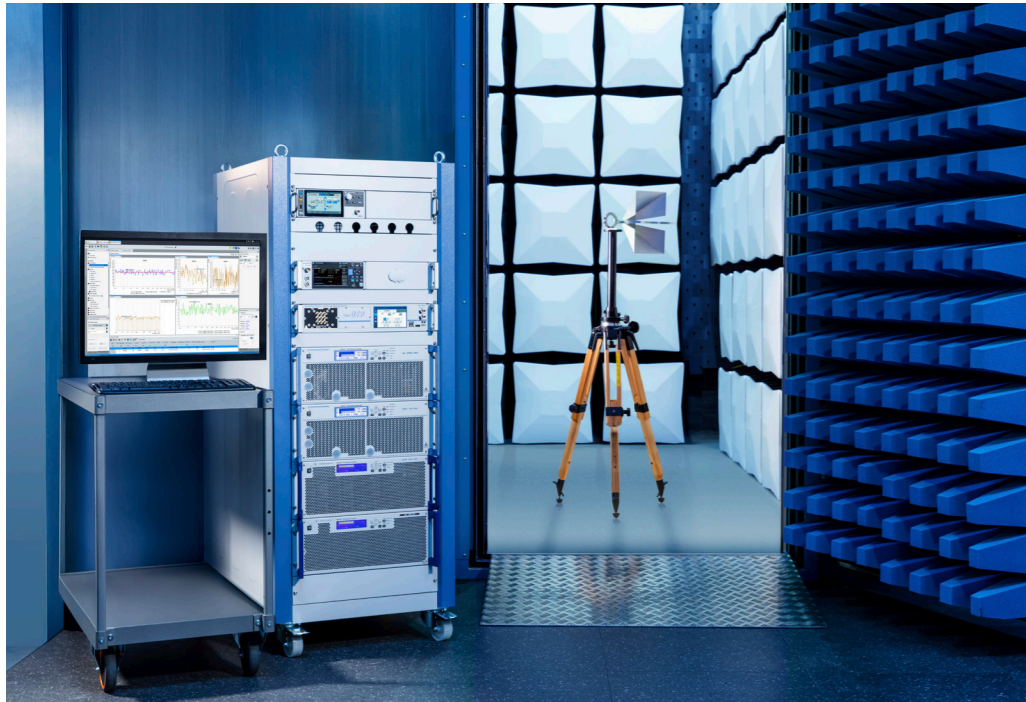
Amplifier system, consisting of 2 × R&S®BBA300 and 2 × R&S®BBA150, deployed in radiated electromagnetic susceptibility tests
