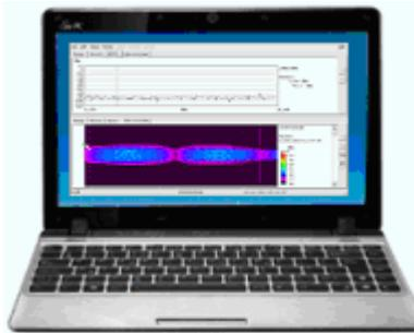
In **Spectrogram** mode ELQ 35 performs spectrum measurements in every second. The results are directly transferred to PC via USB port or indirectly by means of a memory stick when the measurement is completed. Utilizing the large memory capacity and large display of PC the spectrogram program shows the results in form of "Waterfall" diagram in which:
