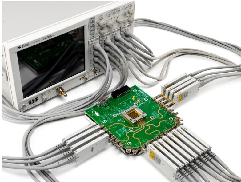
2- to 16-channel TDR/TDT/S-parameter measurement system.
