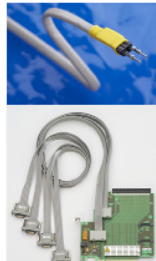
Figure 18. The N4240 Series mid-bus probes feature Soft Touch technology for non-invasive probing
