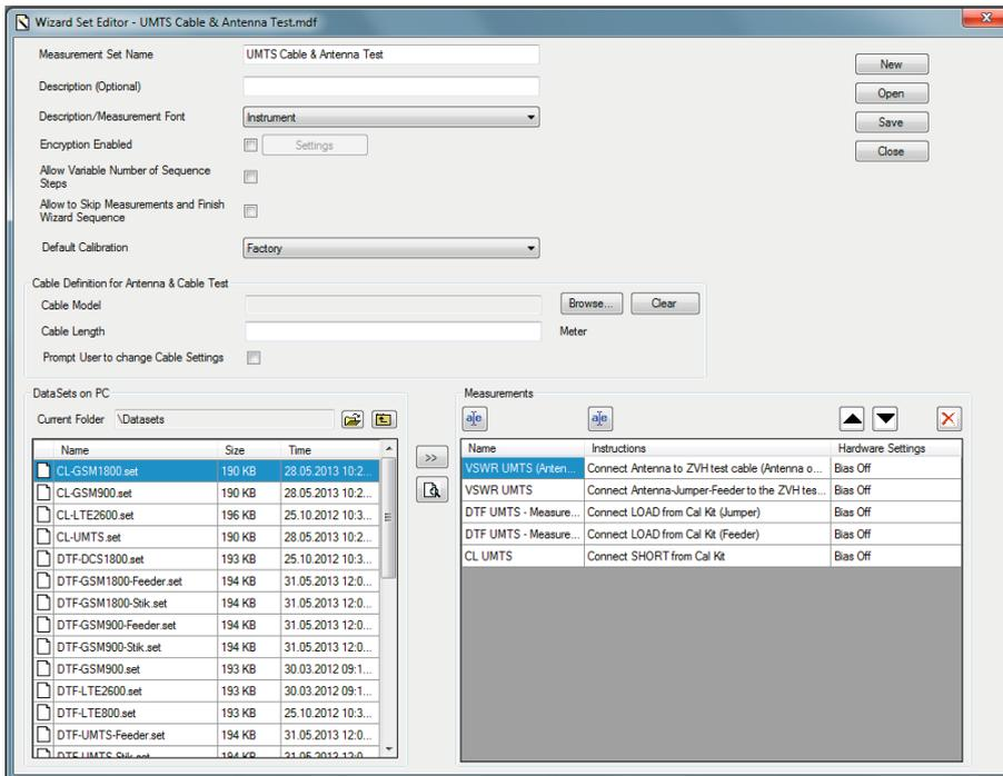
Using the wizard definition editor in R&S®ZVHView, predefined instrument settings can be combined into test sequences on a PC and then transferred to the R&S®ZVH.
