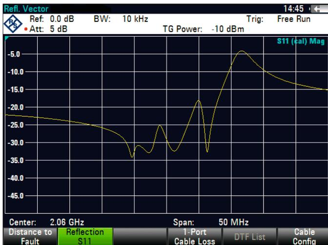
When using an RF jumper cable or an adapter to connect the R&S®ZVH to the DUT, the easy one-port normalization technique compensates the introduced attenuation. The easy one-port normalization is applied on top of the factory calibration and does not require a calibration standard.
