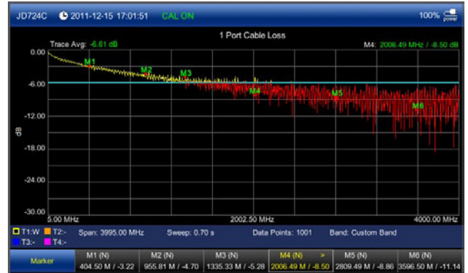
1-Port Cable Loss
