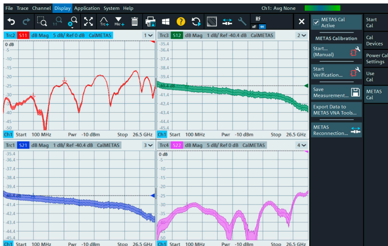
Real-time S-parameter measurements with uncertainty bands
